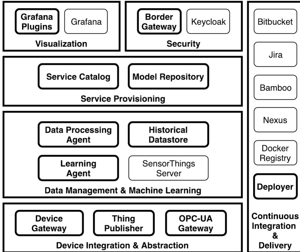
Figure 1. LinkSmart Platform components and DevOps infrastructure.
